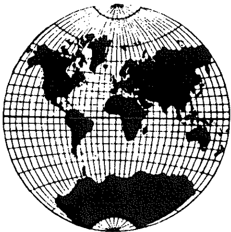
Van der Grinten Projection of sphere within a circle
