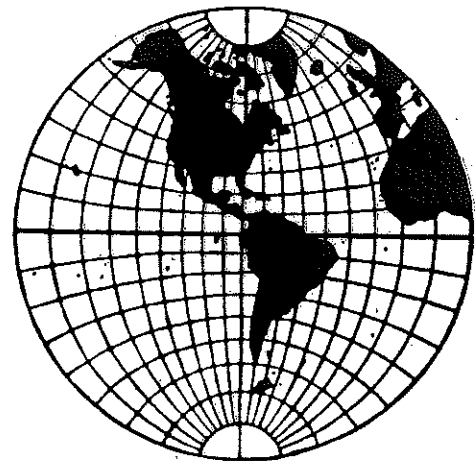
Equatorial case of Stereographic Projection
